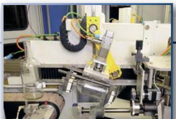
Loading/unloading servo-driven robot arm.
