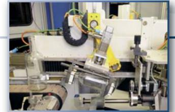
Loading/unloading servo-driven robot arm.
