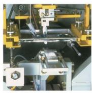
PUSHER AT PRINT STATION to ensure the position of the print with regard to the object height
