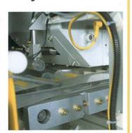
**EJECTION BY SLEEVE** on to belt conveyor for further handling, such as loading into cardboard cartons
