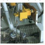
The numeric loading and unloading arm has the advantage of a quick setup by teaching procedure without
