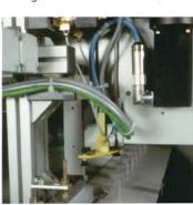
**EJECTION BY SLEEVE** object must be thick walled.
