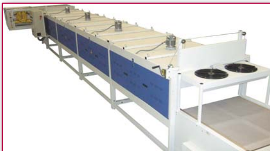
Low temperature oven for traditional (solvent based) ink (250°C)
